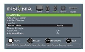
3 Press ▲ or ▼ to highlight Channel Labels, then press ENTER. The CHANNELS · CHANNEL LABELS screen opens with the channel number field highlighted.
