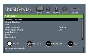
3 Press ▲ or ▼ to highlight Parental Controls, then press ENTER. The Enter Password screen opens.
